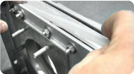
Shimming system for in-line maintenance
